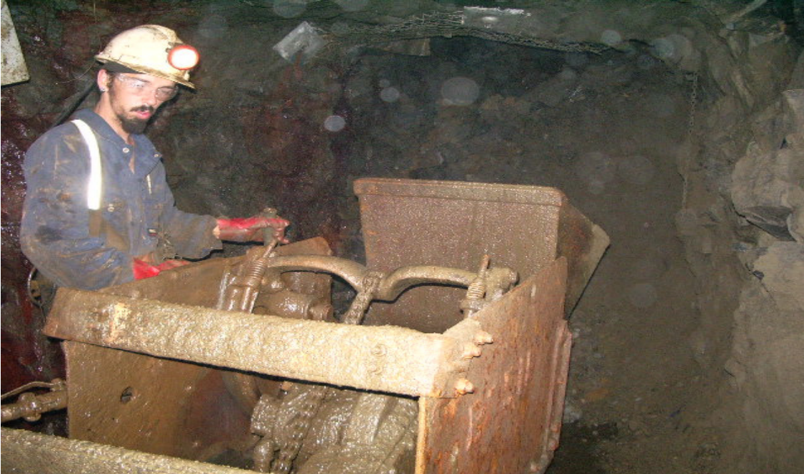
Figure 2 - Derek Mullins operating rail mounted bogger in 3 Level stope drawpoint
